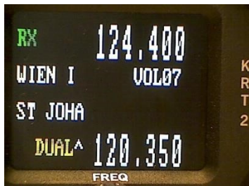
Figure 4: KRT2 active & standby frequencies
